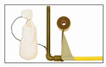
This assembly is not anodeless, it needs external corrosion protection (in the form of an anode bag as shown.) All too often, these elements are improperly applied, or not at all, leaving the assembly open to corrosion, which could lead to leaks. For more information please visit the National Association of **Corrosion Engineers website:**
