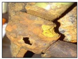
This is an example of unprotected underground fittings that have corroded. Property damage, injury and death could occur if corrosion control elements are not properly engineered.
